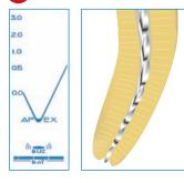
When the apex is reached the V line marked with 0.0 starts to flash and an intermittent beep starts to alert the dentist.
